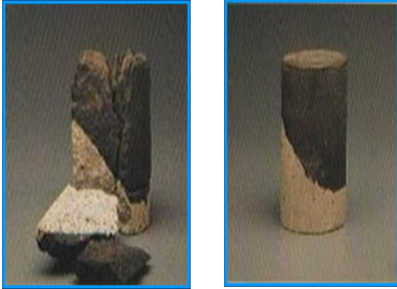
Slant Shear Bond Test
