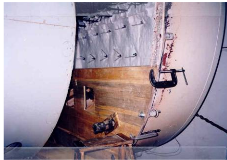
Thermbond Formula Nine is the hot face layer - lower door 8" - shelf is 21" overall depth.
