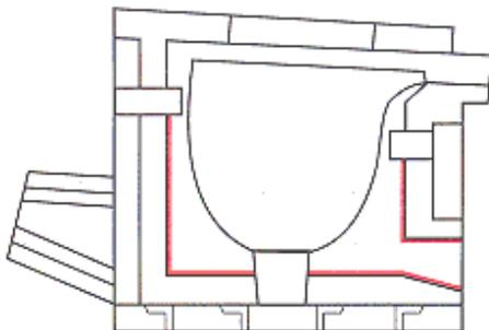
Frequent repairs are necessary due to the damaging effects of high temperature and thermal shock. These conditions cause cracking of the refractory lining and heat losses. Nonvit coated at 2 to 3mm, will eliminate or minimise the problem.
