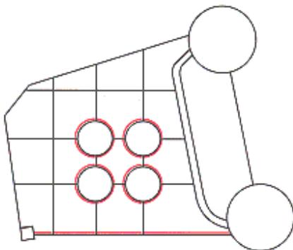
The burner throat is subjected to intense wear and tear due to the effects of high temperature, slagging, chemical attack, erosion and thermal shock. A coating of 2 to 3 mm of Nonvit resists these combined effects on the refractory lining. A coating of 1 to 2 mm on the walls and floors minimises the adhesion of slags and helps in prolonging the life of the refractory life.
