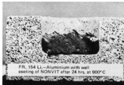
FR, 154 Li.—Aluminium with wall coating of NONVIT after 24 hrs. at 900° C
