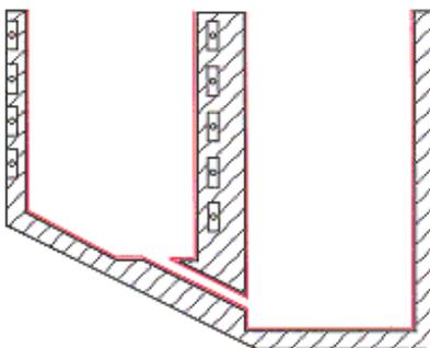
3 mm of Nonvit will seal the refractory against the leaching effects of molten aluminium. 6mm is used to line the connecting channel.
