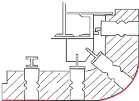
This part of the boiler is subjected to both high temperatures and slag attack from the products of combustion. A coating of 2 to 3 mm of Nonvit on the refractory surface will minimise the effects of spalling, slagging and abrasion.
