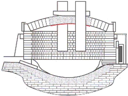
The centre section of the roof is made of either castable or plastic refractory. A coating of 2 to 3 mm of Nonvit will minimise the destructive effect of high temperature and thermal shock, prolonging the life of the refractory.
