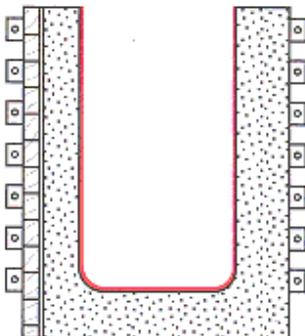
The rammed lining is subjected to chemical attack by molten metal and to cracking and spalling from thermal shock, 1 - 3 mm of Furnascote Nonvit will reduce these effects, extend the life of the furnace and improve the quality of the processed metal.
