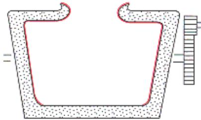
A coating of 2 to 3 mm Furnascote Nonvit on the walls and lips of receivers will prolong the life of the lining.
