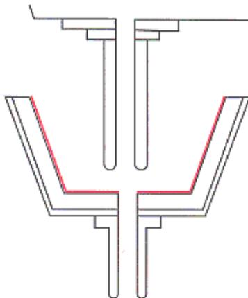
**Steel Tundishes** Frequent repairs and shutdowns are encountered due to the effects of high temperature and thermal shock. A thin coat of 2 to 3 mm Nonvit prolongs the life of the refractory lining.
