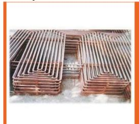
Devised from quality carbon steel or alloy steel seamless tubes, duly stud welded with MS/SS studs, the Bed Evaporator Coils offered by our firm are highly durable in nature. These coils are widely used in FBC type of boilers. Known for their sophisticated designs, these coils are highly acclaimed by the clients in the market. Owing to their optimum performance, resistance to corrosion and reasonable prices, these coils are highly admired by the clients.
