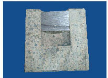
Aluminium corrosion cup test
